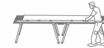
Our products can be cut using diamond discs fitted onto the hand-held electrical grinding machine. The speed of Disc rotation must be high (>10000 RPM) and should have a low feed rate (< 1 m/min). It may be required to cool the disc with water. Recommended discs are the thin types generally used for cutting porcelain stoneware. The surface should be kept on a FLAT base while cutting without any gap underneath
